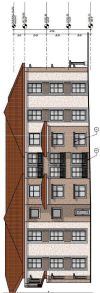
1 BUILDING F ELEVATION - NORTH 1/8" = 1'-0"
