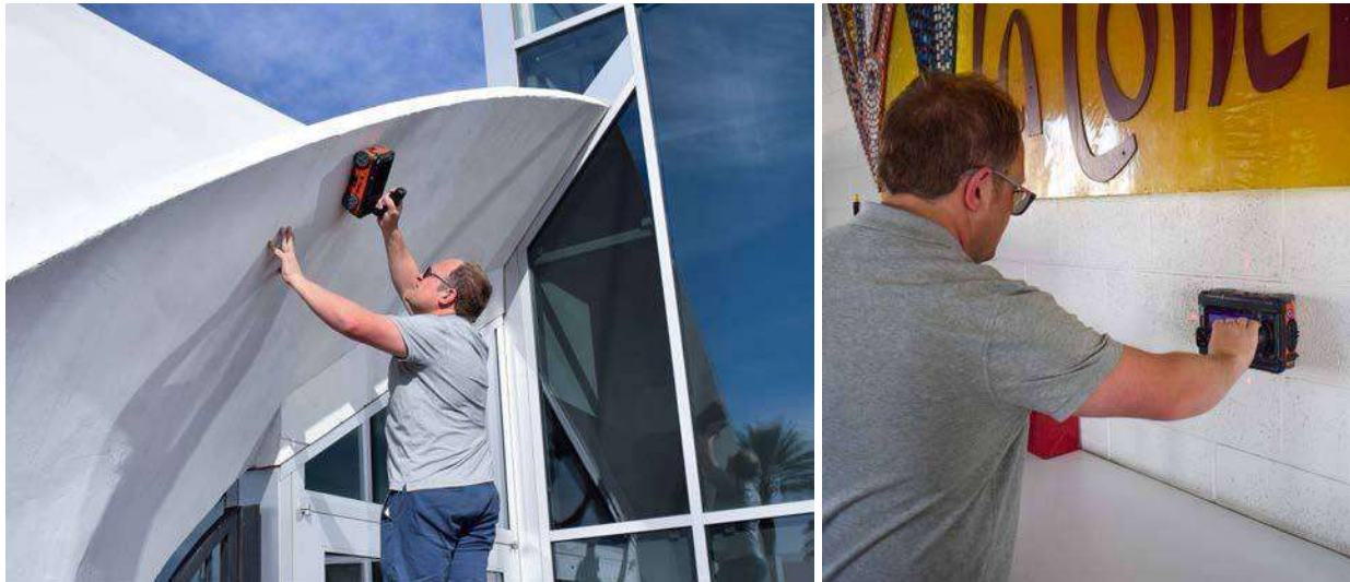
GPR Data Collection: Identifying the reinforcement arrangement within the concrete roof (left) and demonstrating the identification of vertical reinforcement and cell grouting in the CMU wall (right)
