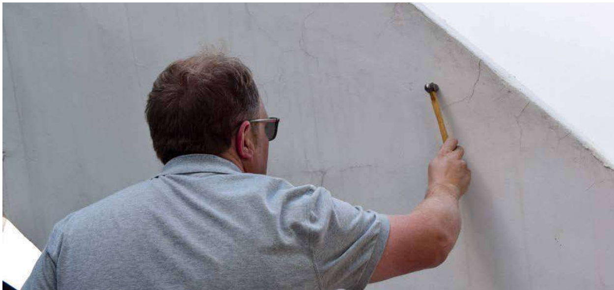
Tap Testing: Cracked surface at south east corner of roof overhang
