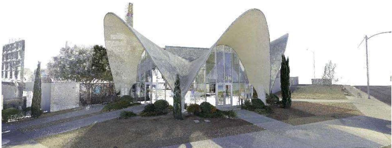
3D Point Cloud: Millions of individual measured points together as a point cloud
