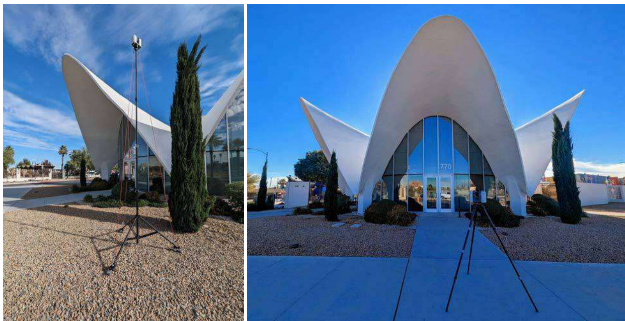
3D Laser Scanning: Laser measurement of The Neon Museum Visitor Center
