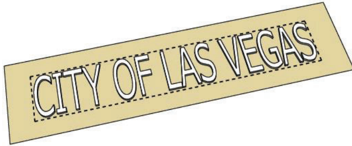
Figure 11 - Sign Area Measurement - Channel Letters
