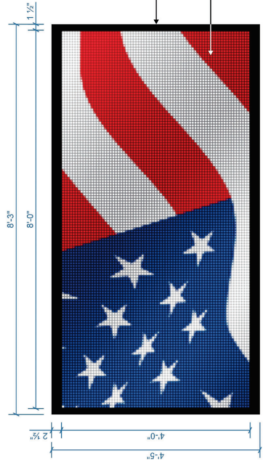
WS-1 S/F WALL MOUNTED LED MESSAGE UNIT QTY: ONE (1) REQUIRED SCALE: 3/4" = 1'-0"
